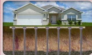
All applications of steel underpins demand the pile to be driven or drilled to competent capacity and/or bedrock and secured to the foundation with brackets capable of bearing at least twice the load necessary to secure the structure. All brackets utilized in residential and commercial projects, by Secure Foundation Systems, Inc., have been tested and approved by the manufacturer.
