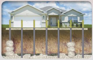
When used for sinkhole remediation, Pressure Grouting is an effective procedure used to seal off the collapsed or eroded limestone surface and fill the voids directly above the problem soils.
